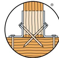
Double-shear nailing use full length Simpson Strong-Tie #9 or #10 screws
